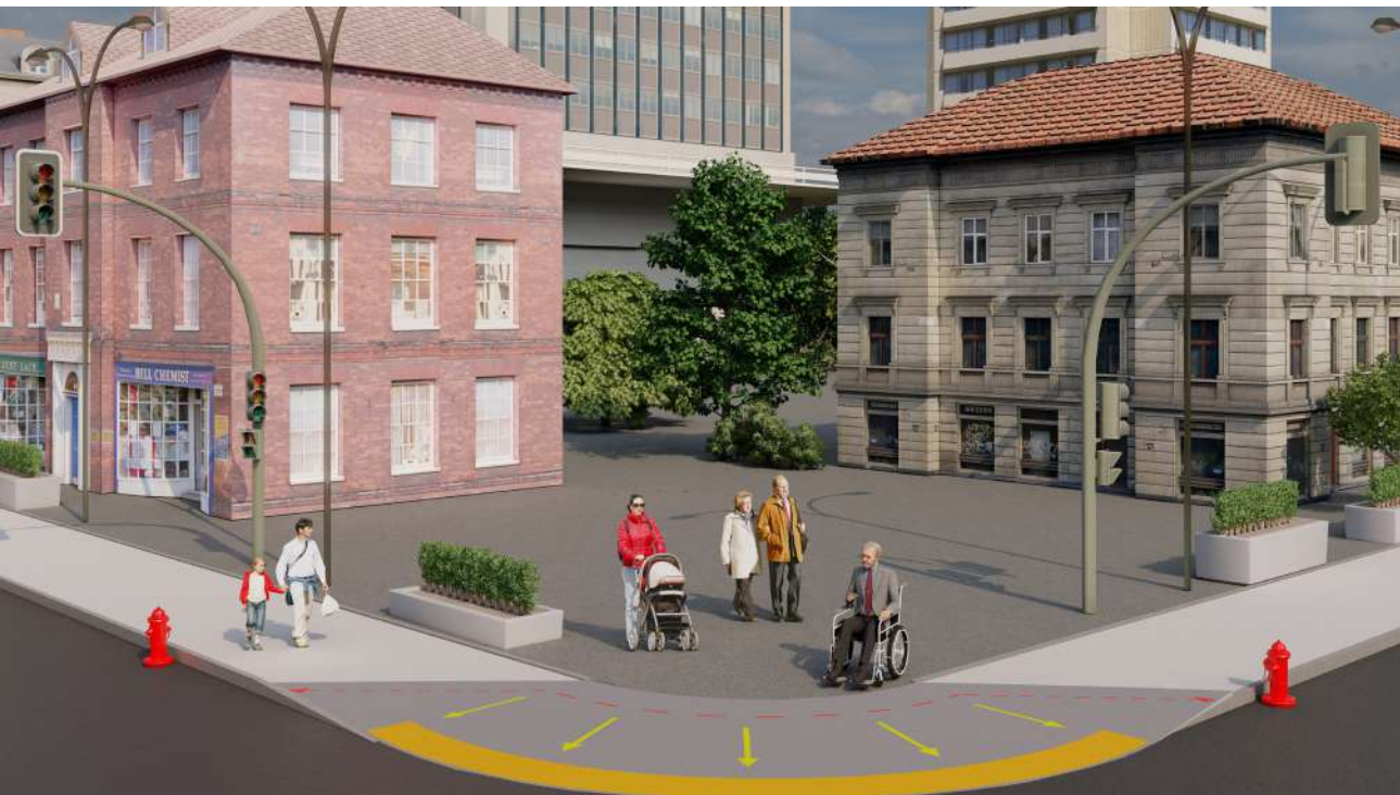
Blended transition with detectable warning surfaces according to the requirements of National Standards of Accessibility
